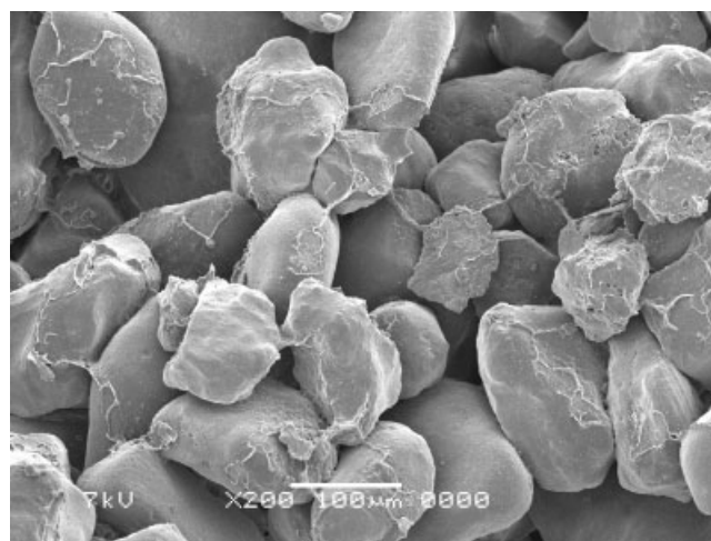
Figure 5 Scanning electron micrograph of a fractured surface of a sample containing 1 wt % polymer prepared by the mixed method.
